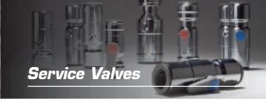
Water Regulations require that you fit a Service Valve on the supply pipe to a tap. mixer or floatvalve. This is to allow for a temporary shut off for future repair or replacement without the need to shut down and drain the whole of the system. Service Valves have a quarter turn mechanism operated by a screwdriver slot, to help avoid unauthorised tampering.
