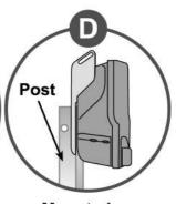
Mounted on a metal fence post using the specially designed slot in the bracket
