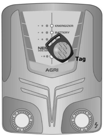
The Nemtek tag is used to toggle the energizer on/off or to toggle the energizer between the low or high power operating state. Hold the tag over the Nemtek logo on the front of the energizer and the energizer will emit a short beep upon detecting the tag.
