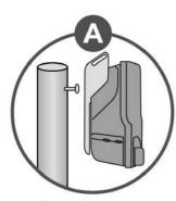
Hanging on a nail hammered into a wooden post (using the slot in the bracket)
