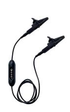
The Easy Fence Tester flashing rate changes with the change of voltage on the fence. The slower the rate the lower the voltage. The intensity of the light remains the same so it can be seen from far irrespective of the fence voltage. It is installed between the earth and live wire to indicate the status and condition of the fence for peace of mind.
